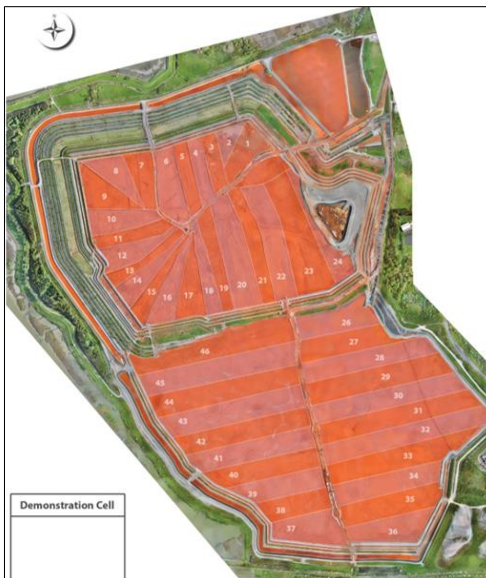
Figure 2.5: BRDA Layered Deposition Cell Layout – December 2020 (Source: Golder, 2021). BRDA Raise
