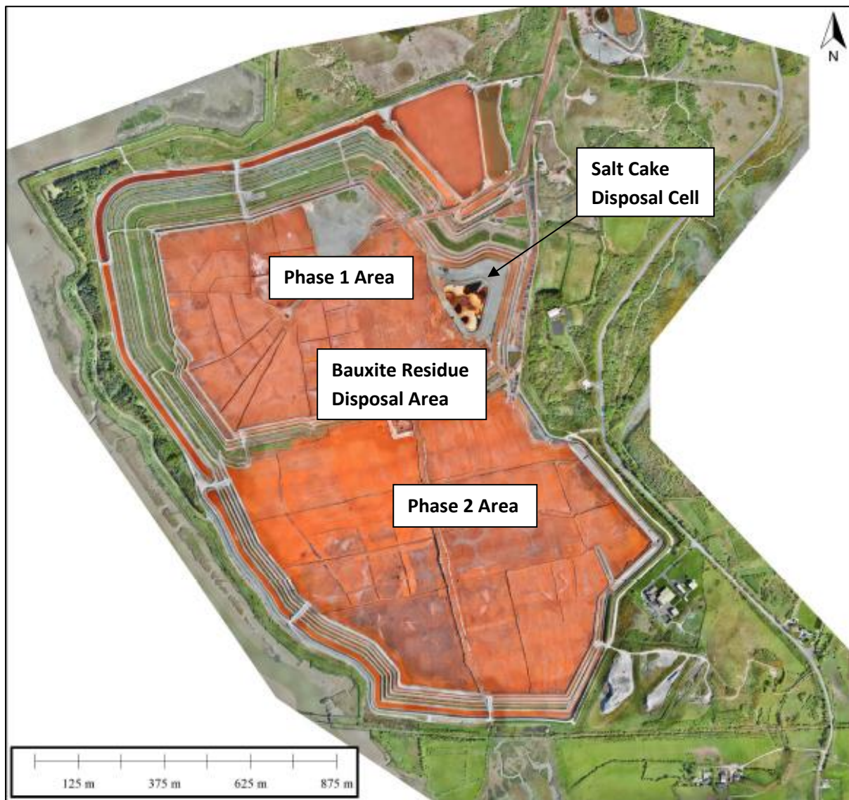
Figure 2.3: Aerial View of part of Aughinish Alumina Site – BRDA (source: Golder Associates).
